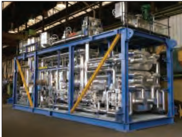
FIGURE 4. A complete membrane system for H 2 is shown here
