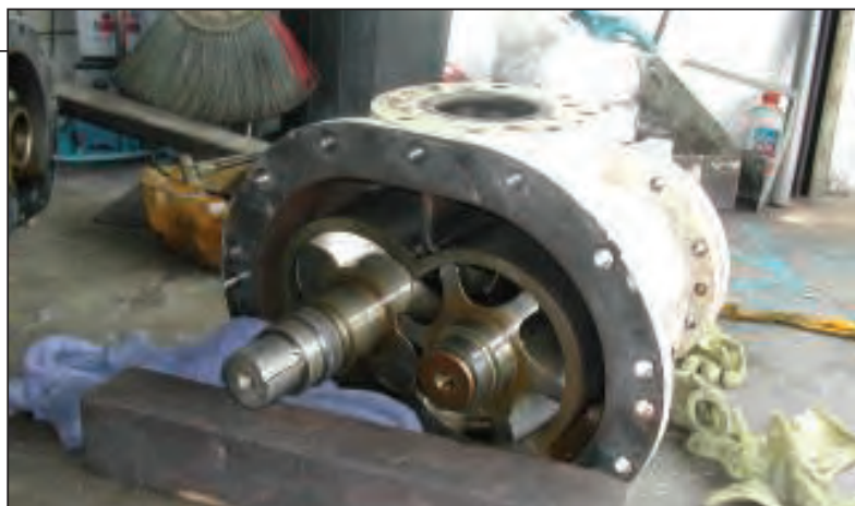
FIGURE 3. The male and female screw rotors, and internal and external casing are shown in this vertically split, oil-injected screw compressor. This machine uses an asymmetric 4+6 screw rotor arrangement (4 male lobes and 6 female flutes), the most common screw profile in various applications. The suction nozzle is located at the top
