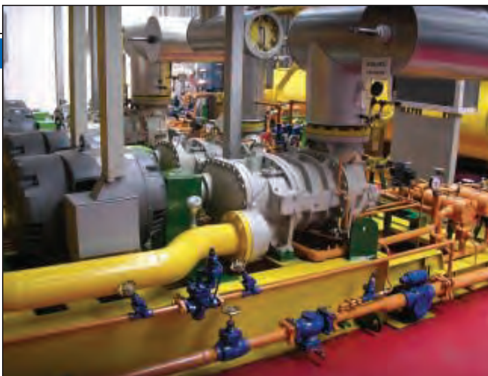
FIGURE 1. This medium-sized screw compressor is driven by an electric motor and installed on a steel frame skid. The top suction and side discharge nozzle arrangement is quite common in mid-size and large machines (typically >0.8 MW). Thermal and pulsation considerations are important when designing and installing the screw compressor's piping arrangement, particularly with regard to the discharge line design. Oil system and auxiliaries are typically included on the same skid
