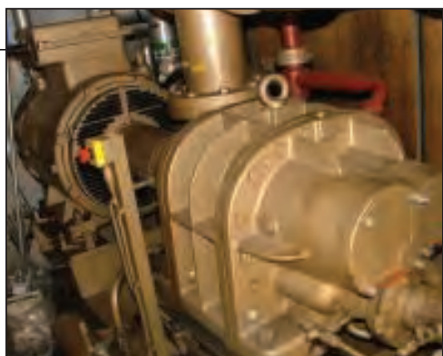
FIGURE 2. In this medium-sized screw compressor, the effects of injected oil result in relatively lower speed (compared to comparably sized, dry-type screw compressors), which enables direct connection between the electric-motor driver and the screw compressor. This eliminates speed-increasing gears, which are usually required in dry-type screw compressors
